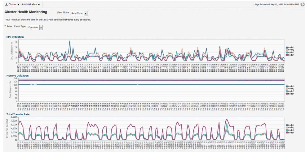
Figure 3-2 Cluster Health Monitoring - Real Time Data
